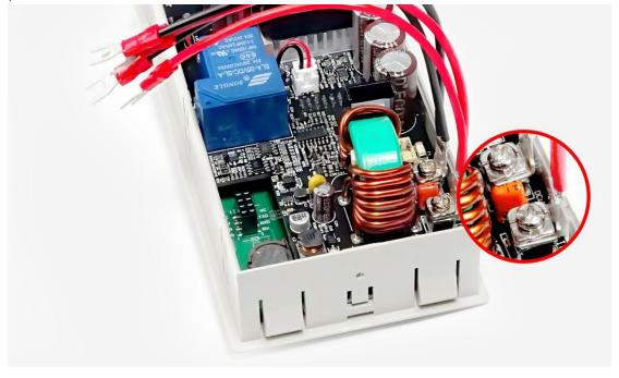
⑤ Assemble the switch power supply: Install the switch power supply on the lower board
